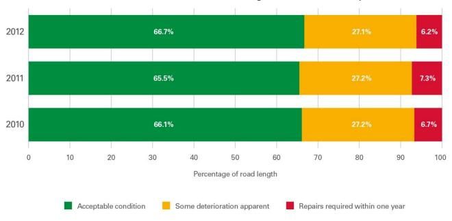
Note: The roads condition survey data is derived from the results of the two most recent surveys, for example the 2012 results in exhibit 1 are based on data for 2011 and 2012. Rather than simply averaging the results from each year, the data collected over the two years is analysed as a single set.
